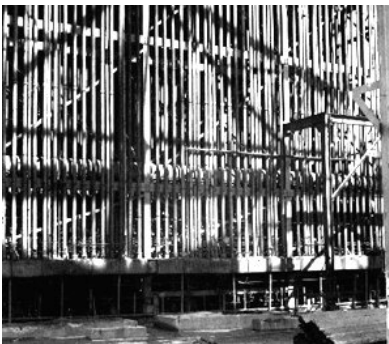
Liquid thermal diffusion uranium isotope separation columns, Philadelphia Navy Yard.
